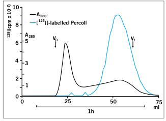
Figure 18. Gel filtration of microsomes obtained from gradients of Percoll containing  $^{125}$ I-labelled Percoll on Sephacryl S-1000 Superfine.  $V_o$  = void volume,  $V_t$  = total volume. (275, reproduced by kind permission of the authors and publisher).
