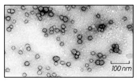
Figure 3. Electron microscopy of Percoll particles. Negative contrast with 1% uranyl acetate at pH 4.6 (21, reproduced by kind permission of the authors and publisher).
