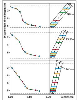
Figure 8. The effect of rotor angle on gradient development using Percoll. Starting density was  $1.065\ g/ml$  in  $0.15\ M$  NaCl. Running conditions:  $30,000\ x$  g for 14 minutes. Colored lines refer to the positions of the colored density marker beads.
