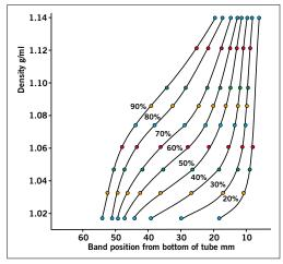
Figure 10. Use of colored Density Marker Beads to show gradient shapes. Dilutions of Percoll as in Figure 9, running conditions: 23° angle-head rotor, 60,000 x g, 15 minutes. Steeper gradients were formed by the greater g-force. (Work from Amersham Biosciences, Uppsala, Sweden.)
