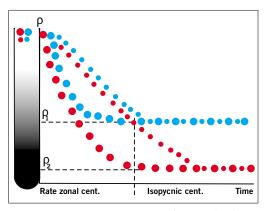
Figure 1. Diagrammatic representation of rate zonal and isopycnic centrifugation. ρ, = buoyant density of the less dense (blue) particles  $\rho_2$  = buoyant density of the more dense (red) particles
