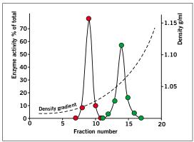
Figure 7. The density distribution of mitochondria from rat liver cells after incubation in iso-osmotic buffer (red) and buffer containing 17.5% albumin (green). Centrifugations were performed in a Beckman 65 rotor (23° angle) for 30 minutes at 40,000 x g. (59, reproduced by kind permission of the authors and publisher).
