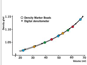
Figure 15. Correlation of recorded densities of a Percoll gradient in 0.15 M NaCl using Density Marker Beads and a digital densitometer (DMA 46, Anton Paar A.G.). Fraction size 2.64 ml, centrifuge MSE Superspeed 75, rotor 10 x 100 ml, angle 18°, 40,000 x g for 60 minutes. (Work from Amersham Biosciences, Uppsala, Sweden.)
