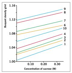
Figure 14. Effects of sucrose concentration on the recorded densities of Density Marker Beads in gradients of Percoll. Numbers refer to different bead types; the exact density of specific lots is printed on the box label. (Work from Amersham Biosciences, Uppsala, Sweden.)
