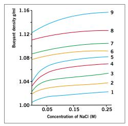
Figure 13. Effects of salt concentration on the recorded densities of Density Marker Beads in gradients of Percoll. Numbers refer to different bead types; the exact density of specific lots is printed on the box label. (Work from Amersham Biosciences, Uppsala, Sweden.)
