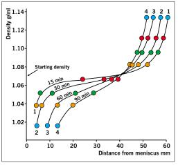
Figure 4. Isometric gradient formation by Percoll in an anglehead rotor,  $8 \times 14$  ml (MSE Superspeed centrifuge) starting density 1.07 g/ml in 0.15 M NaCl. Running conditions:  $20,000 \times g$  for 15, 30, 60 and 90 minutes. Gradient density was monitored by means of colored Density Marker Beads. See Figure 12, page 23 (Work from Amersham Biosciences, Uppsala, Sweden).
