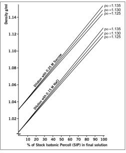
Figure 5. Dilution of Stock Isotonic Percoll (SIP) with iso-osmotic saline or sucrose solution. Po is the density of the Percoll (undiluted). SIP is prepared as described on page 12. The calibration lines shown are for guidance only. For accurate density measurements, refer to the formula given in the text. (Work from Amersham Biosciences, Uppsala, Sweden.)
