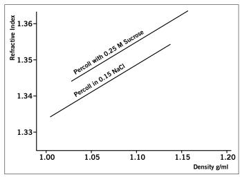
**Figure 16.** Refractive index as a function of density of a Percoll gradient. (Work from Amersham Biosciences, Uppsala, Sweden.)
