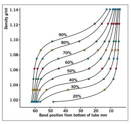
Figure 9. Use of colored Density Marker Beads to show gradient shape. Gradients formed from solutions of Percoll varying from 90% to 20% of stock isotonic Percoll in 0.15 M NaCl. Running conditions 23° angle-head rotor 30,000 x g, 15 minutes. (Work from Amersham Biosciences, Uppsala, Sweden.)
